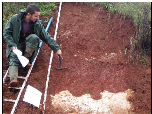
Simone Priori demonstrating polygenesis, including aeolian and colluvial processes, in a typical Terra rossa developed in a doline.
