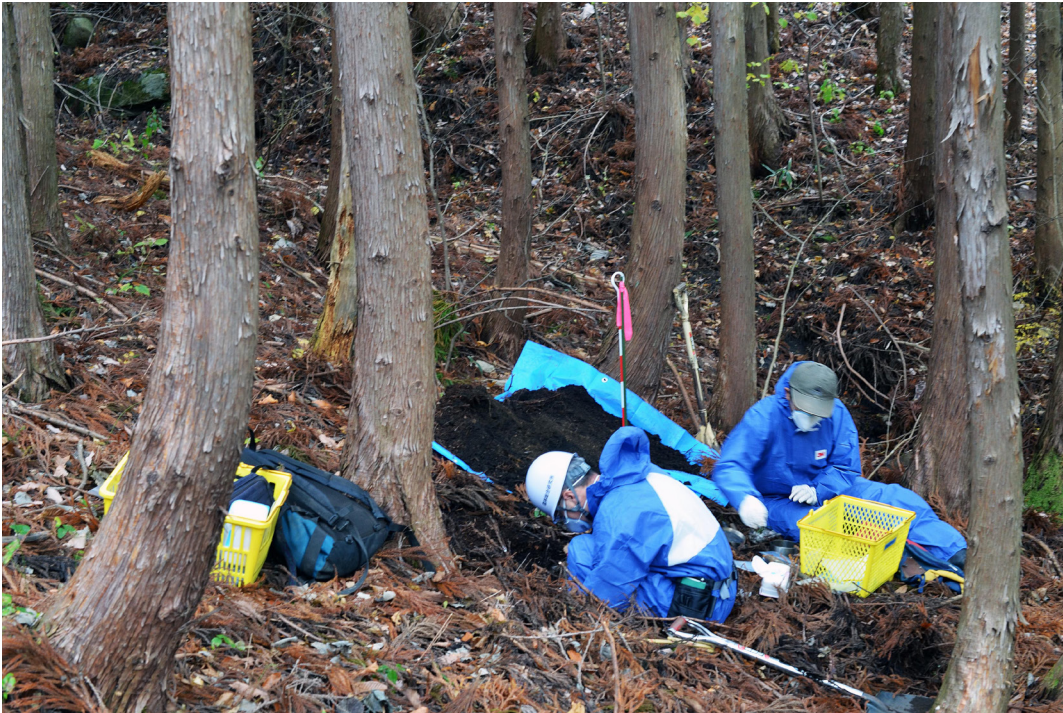
Soil sampling from a contaminated Japanese cedar forest by wearing protective clothing and mask.
